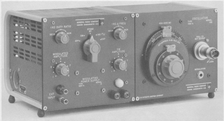
Figure 2. Type 1264-A Attached to Type 1361-A Oscillator.
